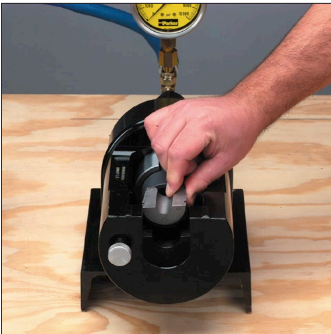
Step 6 Install Lower Die Halve Lubricate the outer conical surface of the Die half. Place the lower Die half in the lower Die Retainer.
