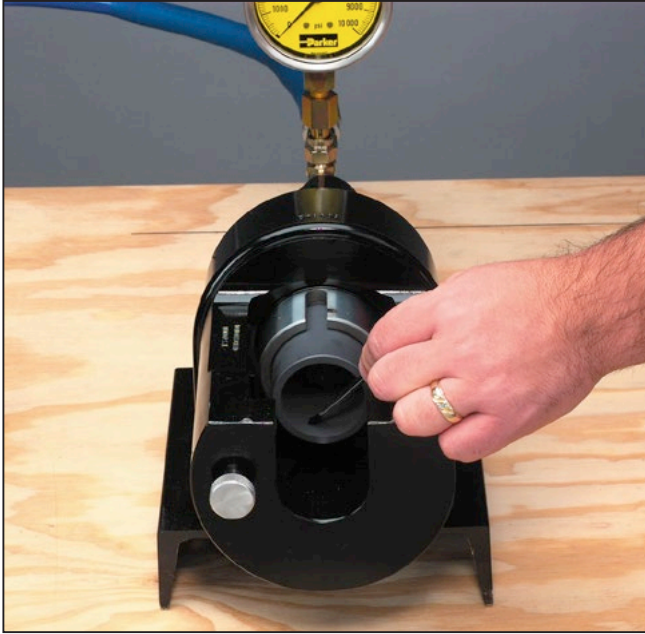
Step 4 Lubricate Surfaces Lubricate the outside surface of the Flaring Cone and the inside surface of the Die Ring with an extreme pressure lubricant (such as STP oil treatment). This will prevent galling and adhesion of components during operation.
