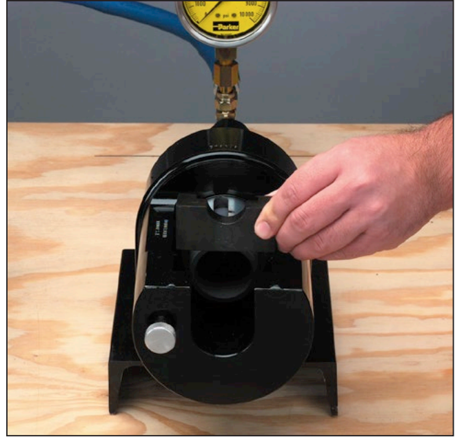
Step 5 Lower Die Retainer Install the Lower Die Retainer into the Hydra-Tool by placing into the slot located near the front of the Hydra-Tool. Assure that the slot in the retainer is facing upward.
