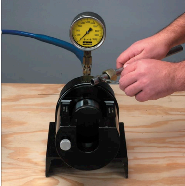
Step 6 Lubricate Ferrule Lubricate leading outer (bite) edge of ferrule with lubricant. Lubrication reduces wear on the die and reduces friction to ensure that all force is available to preset the ferrule.
