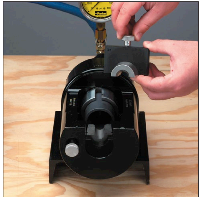
Step 7 Install Upper Die Install the Flaring Die half with the threaded hole into the upper half of the Die Retainer Assembly with the knurled thumb screw. Secure the die in place by turning the knurled thumb screw clockwise.
